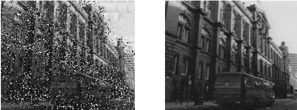
Figure 4: a) An image from a video reconstructed from both the base and enhancement layer. Note the excessive amount of quantization error accumulation, resembling noise. b) Image from a reconstruction using only the base layer, which exhibits poorer quality but no quantization error accumulation.
