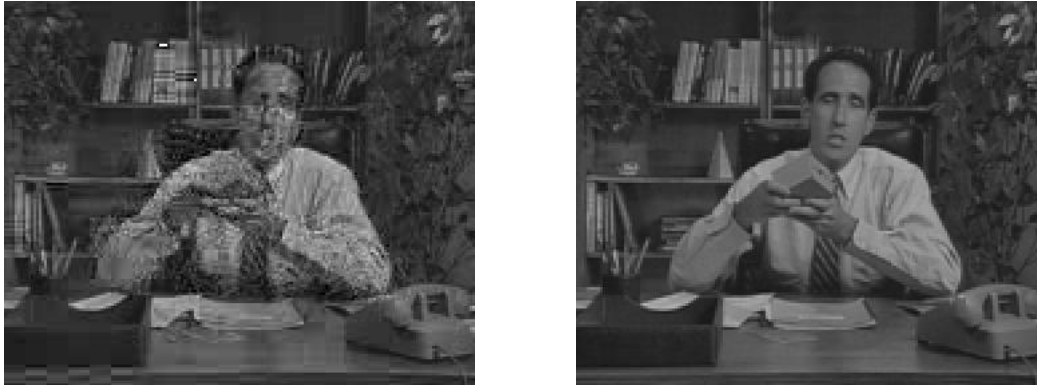
Figure 6: Reconstructed videos from the encoder in Fig.5 a) Using only the base layer, drifting, the trailing left behind by the moving arms and hands, is very noticeable. b) Drift-free reconstruction results when the enhancement layer is also used.
